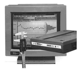
Analog gage ports provide excellent resolution through a 12-bit (plus sign) A/D converter. Data from a column gage with a full-scale resolution of  $\pm$  .010 will resolve to 2.5 millionths of an inch. The MGI with analog capabilities also provides...
